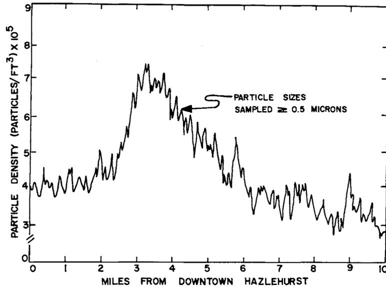
FIG. 6. Smoke plume cross section made while flying in a northerly direction from Hazlehurst, Georgia, and approximately 10 miles downwind from the Lumber City prescribed burn.
