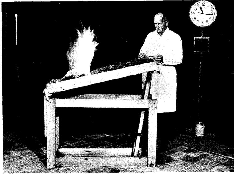
FIG. 1. Environmental conditions are closely controlled inside the combustion room at the Southern Forest Fire Laboratory. Illustrated here is one method used for simulating head fires and backfires.
