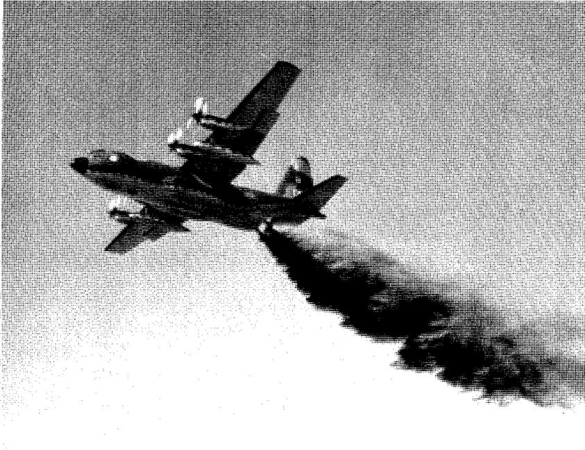
Fig. 3. One of the most recent advances in fire control technology is the large, multi-engined air tanker. Here 3000 gallons of chemical fire retardant is being dropped from a pressurized system flown in a Lockheed C-130. U.S. Forest Service photo.
