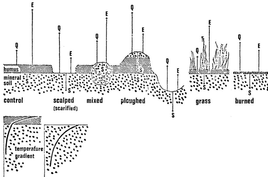
FIG. 3. Heat balance patterns after selected types of soil treatment.
