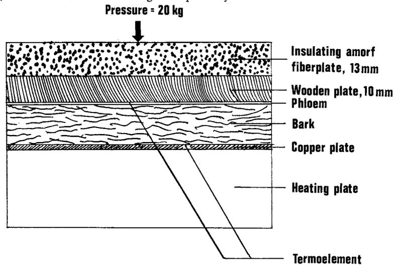
FIG. 7. The laboratory device for measuring thermal conductivity of bark.
