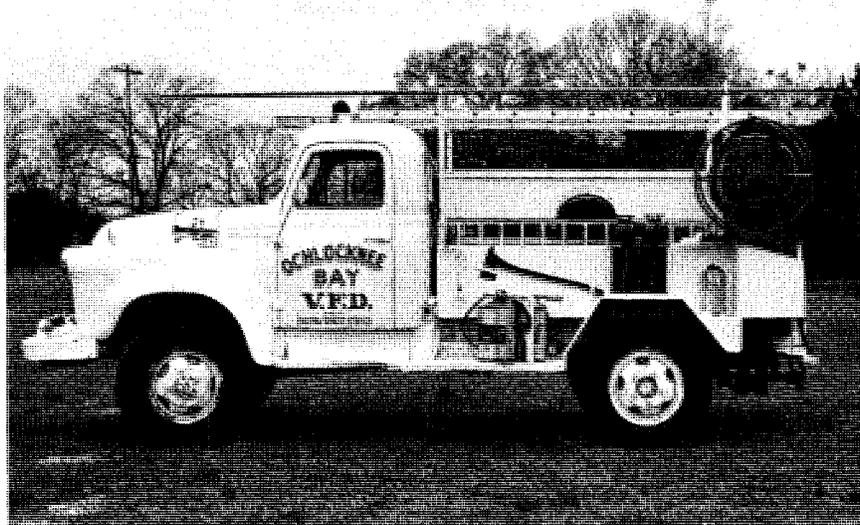
FIG. 2. Florida Forest Service on lease arrangement made this truck available to a Volunteer Fire Department. The volunteers equipped it with a 500 gallon tank and pump powered from the truck's power take-off.
