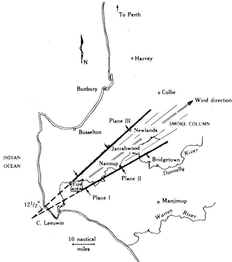
FIG. 2. Spread of smoke from a large prescribed fire in Southwestern Australia. The lateral extension of the column was determined by aircraft traverses through the smoke at Planes I, II, and III as shown: the corresponding angle of spread, as measured in this way, was  $\sim 12\frac{1}{2}^\circ$ .
