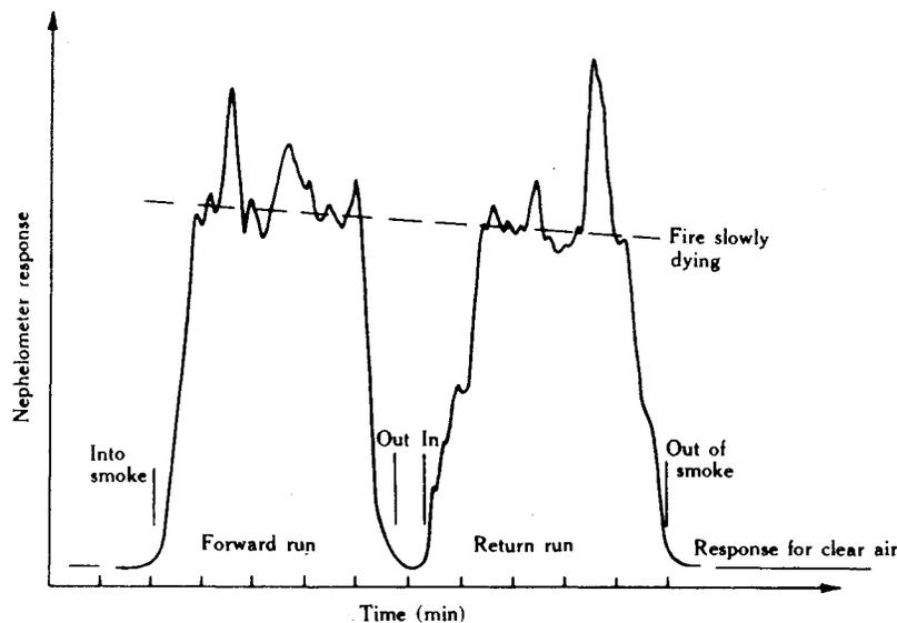
FIG. 1. Typical nephelometer trace obtained during flight through a smoke column: numerous smoke "eddies" are clearly evident, both within the column and at the edges of the smoke.
