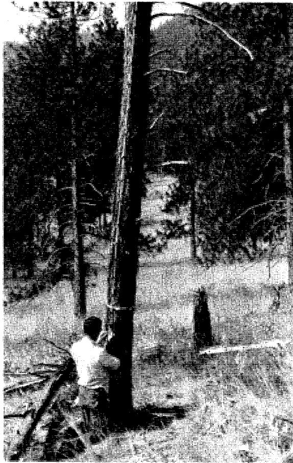
FIG. 11. Live ponderosa pine wired with three 3.6-m.-length strands of 50-grain detonating cord, parallel to tree's grain and against dry outer bark surface, August 1969. (USDA Forest Service photograph by author.)
