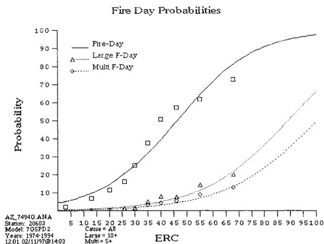
Figure 6. Probability of a fire-day, large-fire-day, and multiple-fire-day as a function of Energy Release Component (ERC) for the Tonto National Forest in Arizona, output from the FIRES: Fire Information Retrieval and Evaluation System. An analysis of the relationship between fire activity and fire danger rating indexes can be used to define critical fire danger levels to support an assessment of the risk of escaped prescribed fire.
