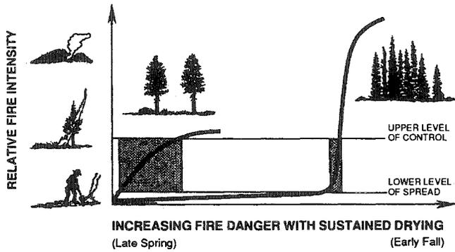
Figure 1. Fire dynamics diagram showing the change in fire potential as a function of sustained drying. A comparison of prescribed burning windows between a ponderosa pine type and a subalpine fir type (from Williams and Rothermel 1992).
