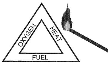
Figure 2. Fire fundamentals triangle illustrating the factors that must be in place for combustion to occur. This applies to a burning match as well as a crown fire.
