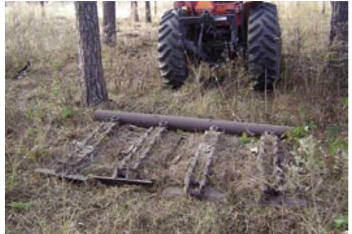
*A simple drag built from tracks and attached using a cable, and below, a drag fitted to a 3-point hitch.*
